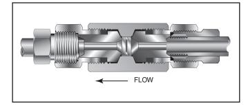
Parker Autoclave Engineers Dual-Disc Line Filters are utilized in numerous industrial, chemical processing, aerospace, nuclear and other applications. With the dual-disc design, large contaminant particles are trapped by the upstream filter element before they can reach and clog the smaller micron-size downstream element. Filter elements can be easily replaced.
