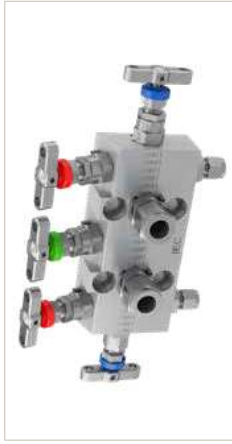
5-valve direct mount manifold for differential pressure applications having inlet and vent connections provided through the use of PTFree connect™ tube fittings.
