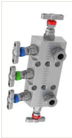
5-valve direct mount manifold having the Parker superior advantage input connections provided through inverted tube fitting connections. Vent can also be specified as threaded or PTFree connect™.
