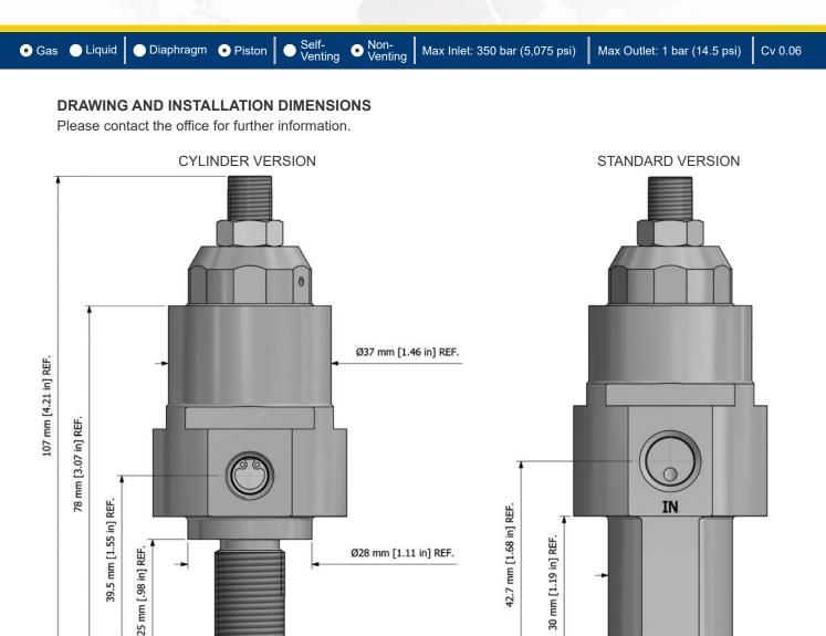
CONNECTION SIZE EXAMPLE OF '1' & '2' (SEE RIGHT): 1 – 2 x 1/8" NPT High Pressure & 2 x 1/8" NPT Low Pressure
