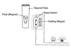
Caution must be taken when mounting multiple alarmed meters. Close proximity may cause interference with alarm signal.
