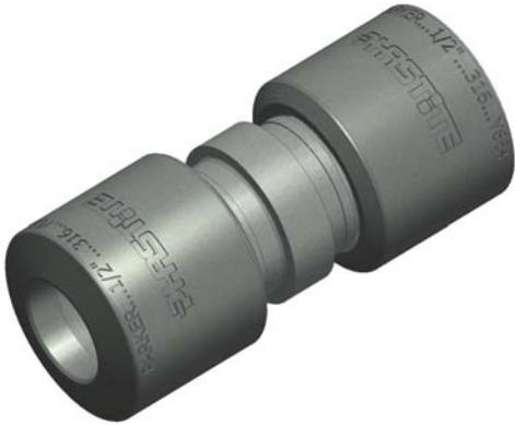
Phastite® permanent connectors use patented seaming technology to provide a unique permanent joint onto standard ASTM A269 tubing. The robust design ensure leak free performance in the most demanding of applications, and yet can be assembled in seconds with no manual effort.
