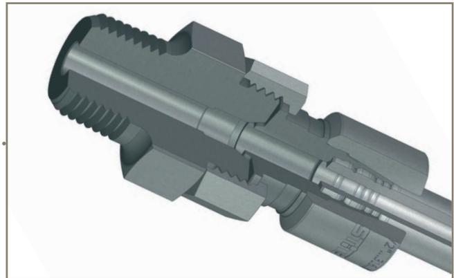
A mating conical arrangement provides leak tight sealing at the breakable joint, while correct assembly is ensured by a metal to metal stop face, without counting turns or monitoring torque levels.
