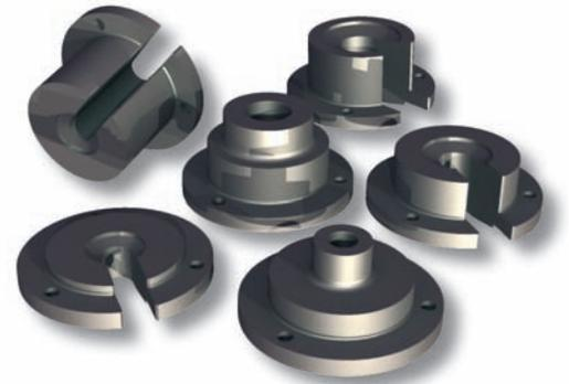
Inserts for assembling termination style Phastite® can be ordered by using the code **PH-M##-TERMININSERT-T\$**, where **##** represents the Phastite® size and **\$** represents the tool size. In the case of 8mm Phastite® Termination ends, the M10 insert should be used.
