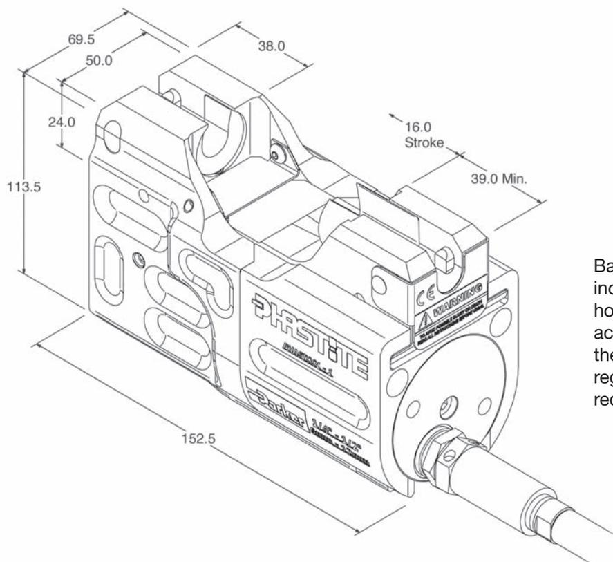
Basic dimensions of this tool are included for planning installations however for installation with limited access available it is advised to consult the factory for more information regarding jaw movement and access requirements.
