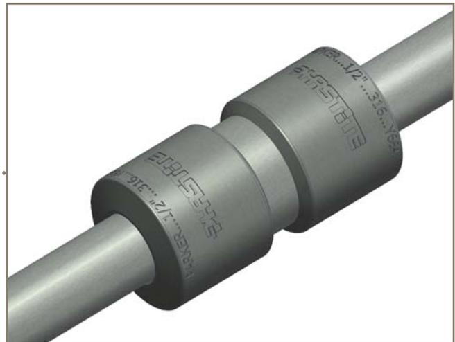
A series of formed ridges makes contact with the tubing surface uniformly to create both a multiple seal and a secure mechanical grip.
