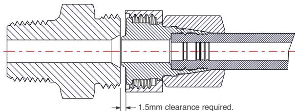
The ability to 'break' and 'remake' the joint is dramatically enhanced by the virtual zero clearance of the design. Allowing the joint to be completely disconnected and removed without large pull out being required.
